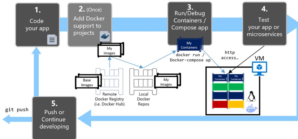
Figure X-XX. Simplified workflow when developing with Visual Studio
