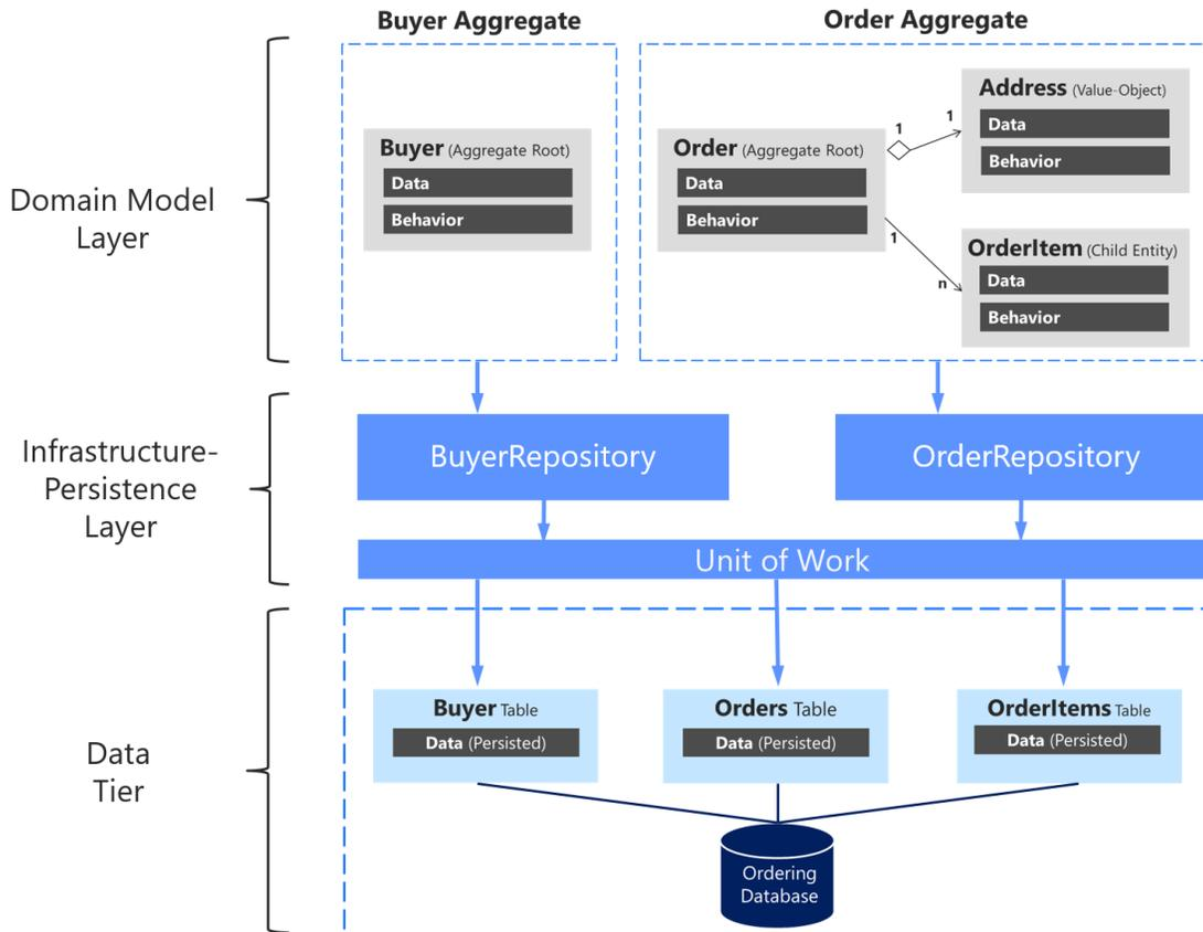
Figure X-XX. Relationship between Repositories, Aggregates and Database Tables
