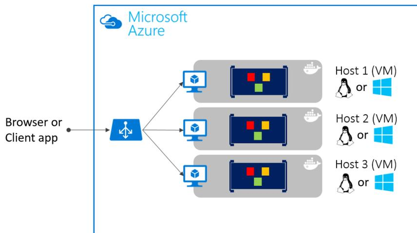
Figure 5-3. Multiple hosts scaling-out a single Docker application
