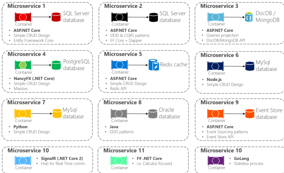
Figure 6-3. Multi-architectural patterns and the polyglot microservices world
