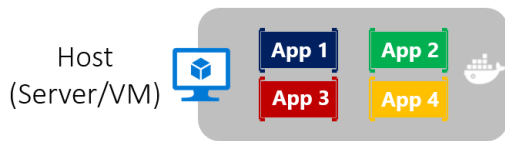
Figure 4-2. Monolithic approach: Host running multiple apps, each app running as a container
