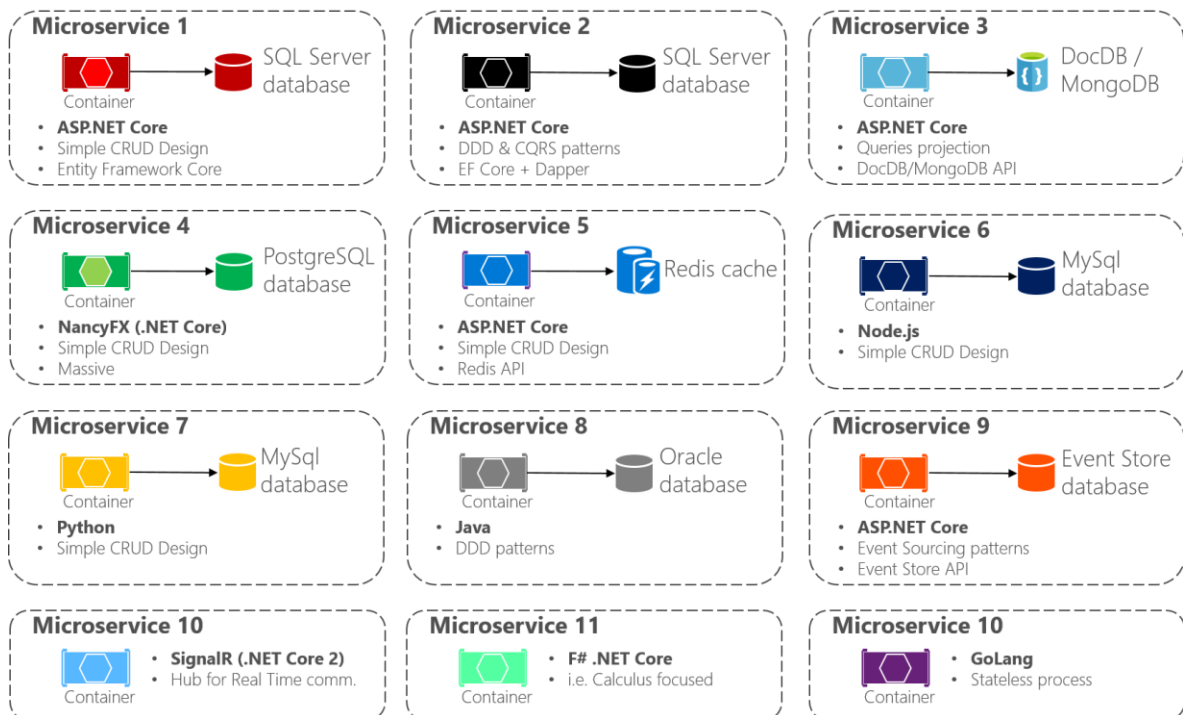
Figure 8-3. Multi-architectural patterns and the polyglot microservices world
